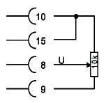
Input of set value only for voltage, pin 15 (set value current) connected to +10V reference, limiting the current to the maximum value by this.
