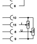
Link between pins 12 and 6 to release the output. 0 - 10V set value input at pins 8 (voltage) and 15 (current). The graphic shows the generation of set values by voltage divider potentiometers, using the internal reference at pin 10. External generation of set values is also possible by digital analog converters or other signal sources.
