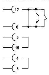
A Link from pin 12 to pin 6 releases the output, a disconnection between these pins locks it. The link can be made by switch, relay contact, wire link, transistor or opto-coupler output (care for correct polarity in the last two cases). Links between pins 15 and 5 and also between 8 and 4 forward the signals of the front plate potentiometers.
