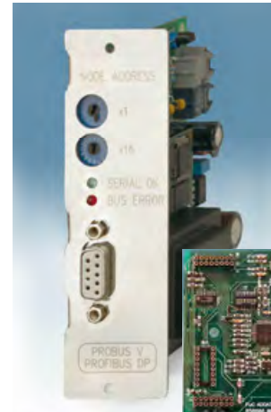
Design Example Interface converter Profibus DP
