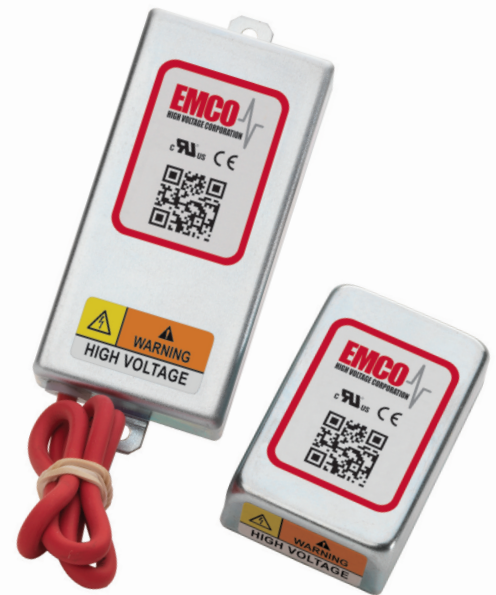
Figure 1: High voltage power supplies designed for sensitive detector biasing employ low noise circuit techniques, magnetically shielded transformers, and plated steel enclosures for low ripple, EMI and RFI.
