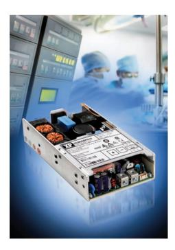
The drive for smaller power supplies goes hand-inhand with a need for greater efficiency. There's a direct relationship here because the smaller the power unit, the smaller the area available for dissipating heat through conduction and convection. Through both measurement and calculation, XP Power has developed a guide to the maximum power loss that can be tolerated for a given size of power supply, based on using convection cooling.
