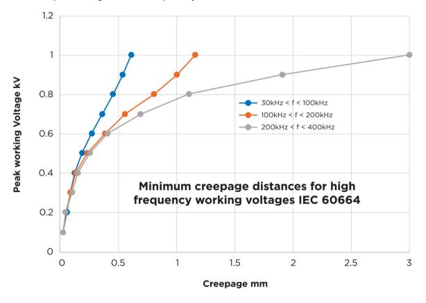
Figure 1: Graph - Creepage distances depend on frequency, not just voltage.
